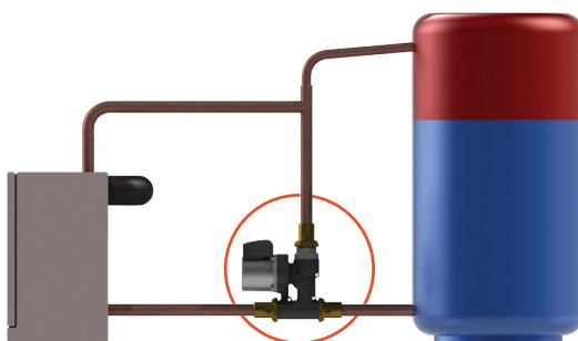
Laddomat 20 is installed between the boiler and the tank.
